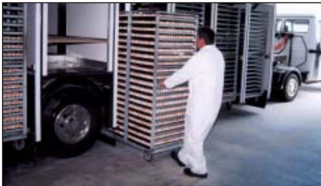
This egg collection truck has been specifically designed for the farm, maintaining the eggs in a temperature controlled environment on route to the farm's egg store.
